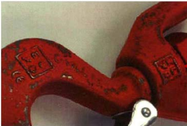
Figure A-30: Swivel Hook – Red Counterfeit
