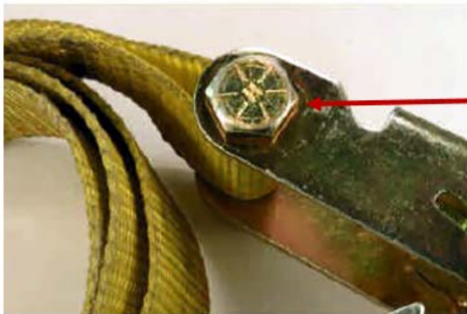
Figure A-15: Ratchet Strap Tie-Down – Counterfeit
