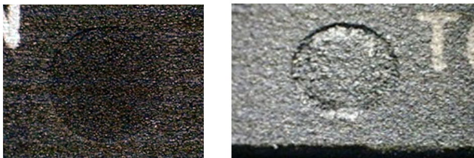
Figure 7: Indents that have been filled in with “blacktopping” material
