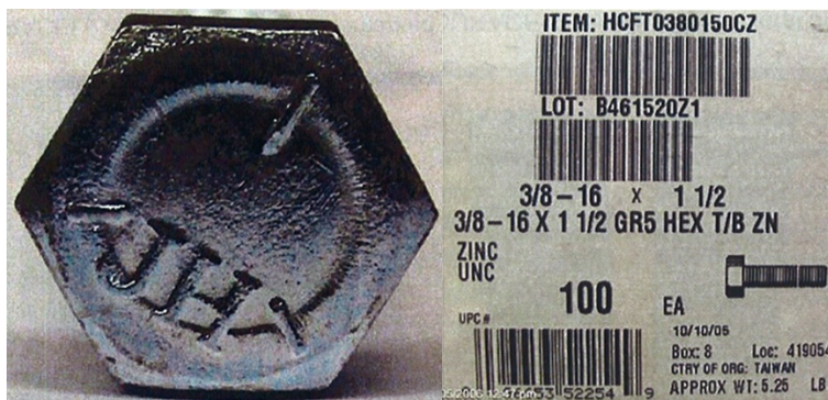
Figure A-4: Jinn Her “JH” Grade 5 Hex Bolt from the West Valley Demonstration Project
