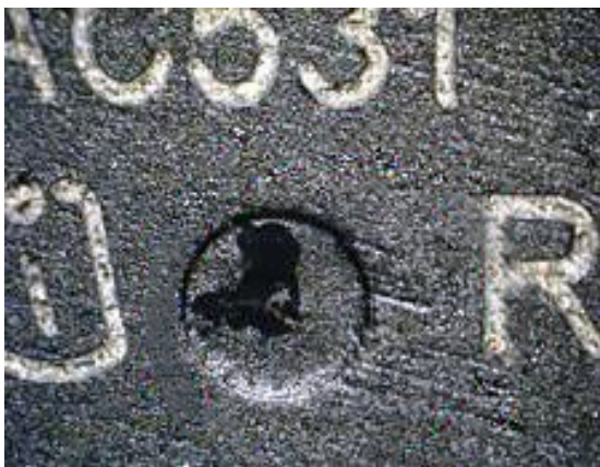
Figure 9: Parts with Directional Sanding Markings
