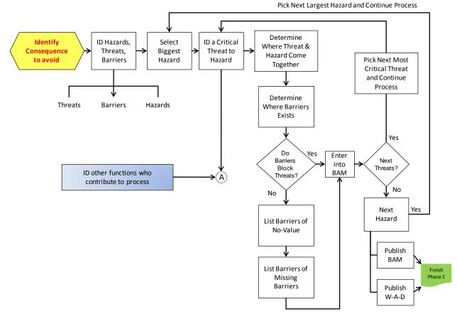
Figure 1-5: Barrier Analysis Process to Capture "Barriers-As-Done"
