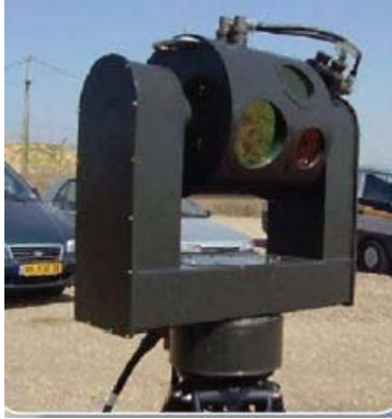
Figure 1. Stabilized Panoramic Intrusion Detection and Recognition System
