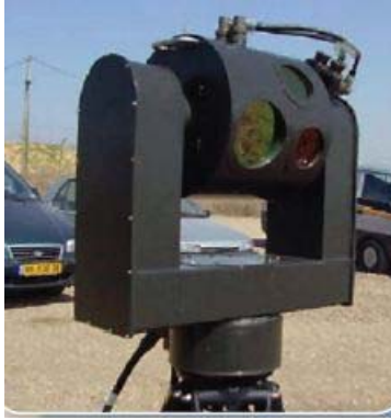
Figure 1. Stabilized Panoramic Intrusion Detection and Recognition System
