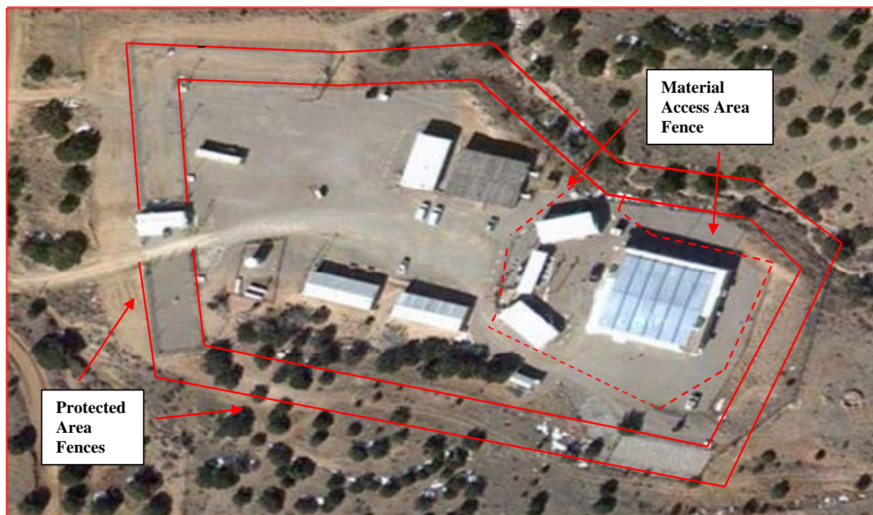
Figure 10. Layout with Perimeter Fences and Protected Area Fences Added
