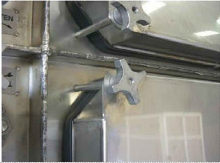
Figure 4.30: Access Door Hand Knobs
