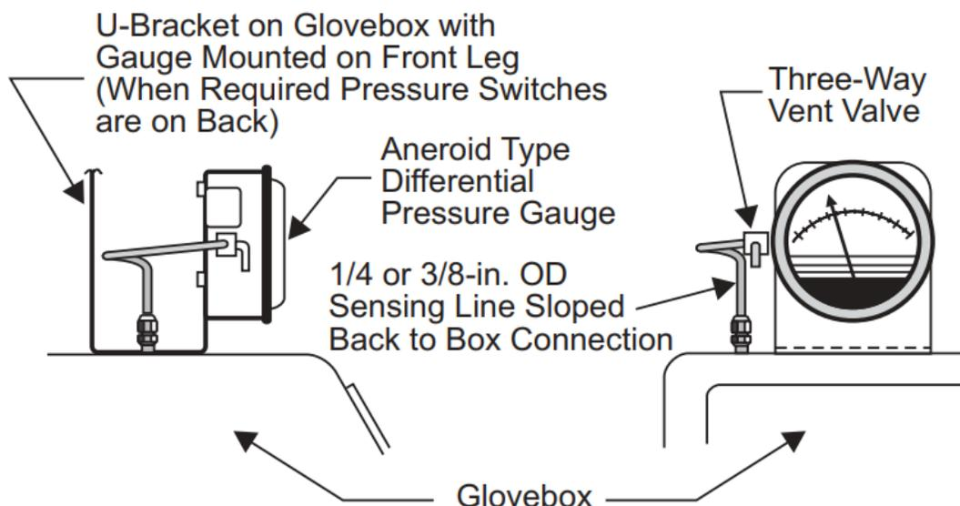
**Figure 4.19: Typical Local Mounting for Differential Pressure Gauge**
