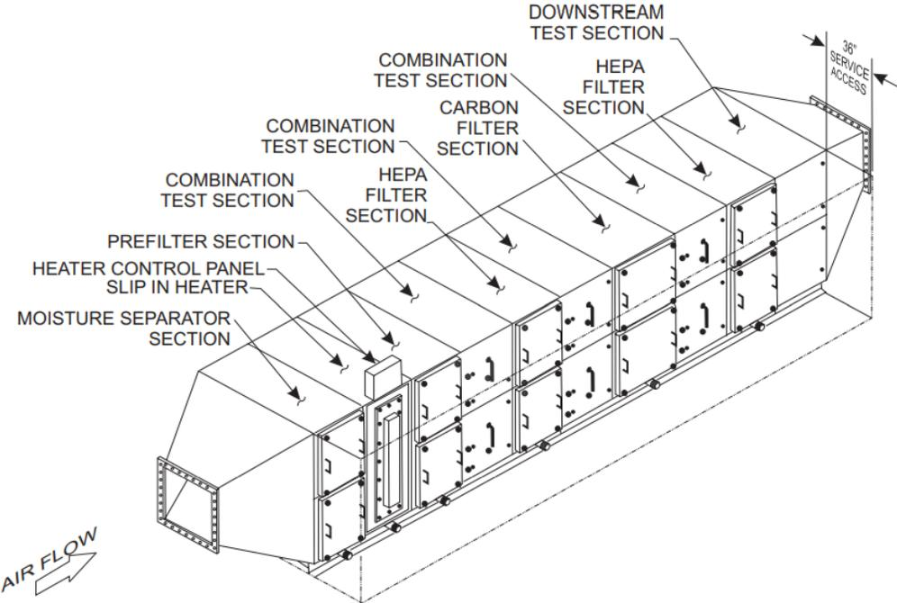
Figure 4.66: Desirable Air Cleaning Housing Features (b)
