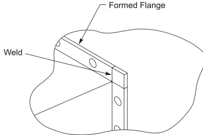
**Figure 4.77: Acceptable Formed Flange**
