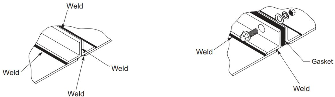
**Figure 4.76: Acceptable Transverse Joints**
