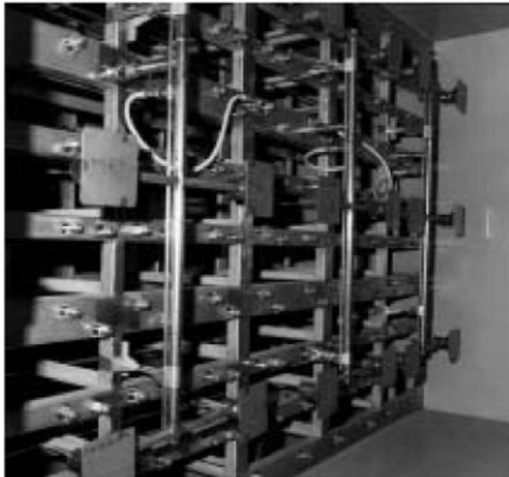
**Figure 4.54: Absorber Mounting Frame with Test Section Manifold**
