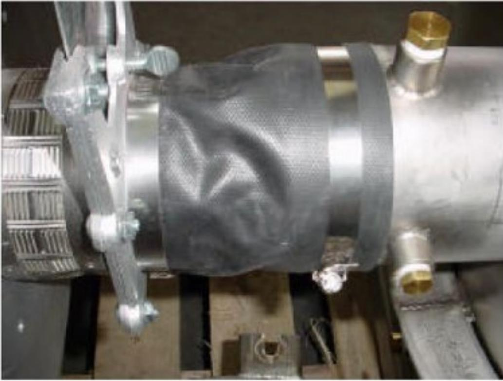
**Figure 4.35: Flexible Connection**
