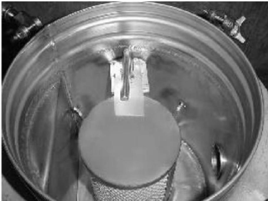
**Figure 4.40: Clearance Between Radial Flow Filter and Housing**
