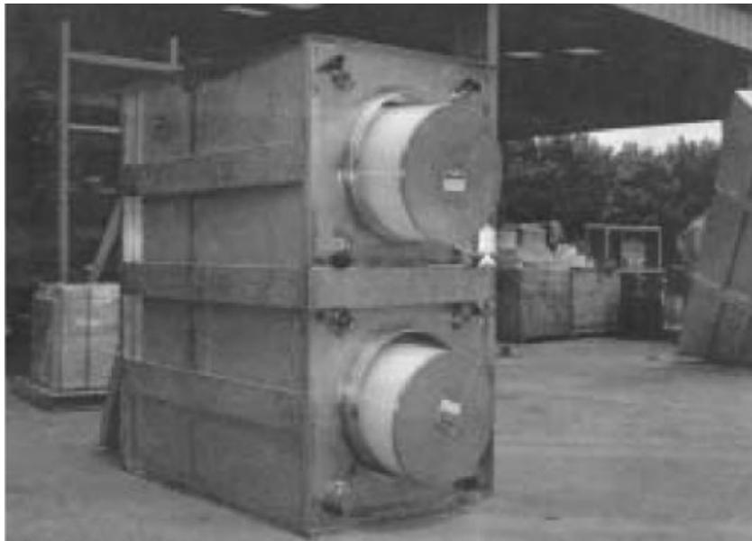
**Figure 4.72: Side Access Housing**
