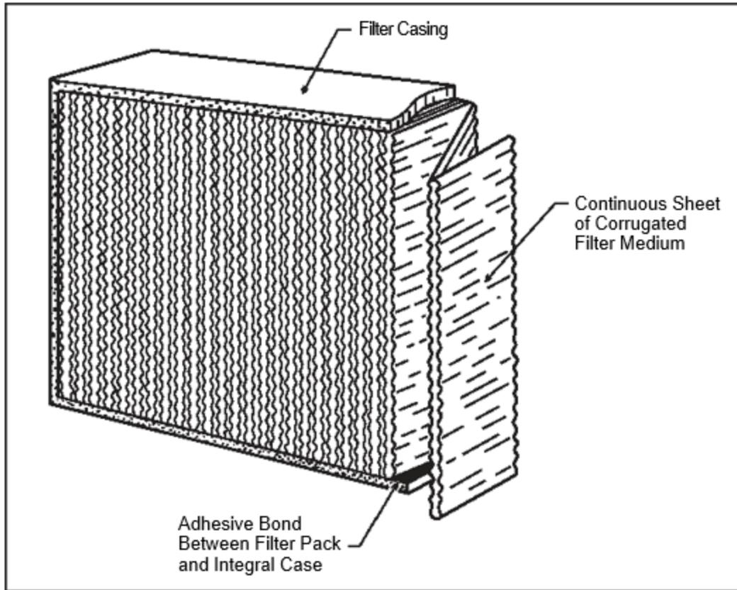
**Figure 4.4: Separatorless Style Filter – Type C Filter Pack**
