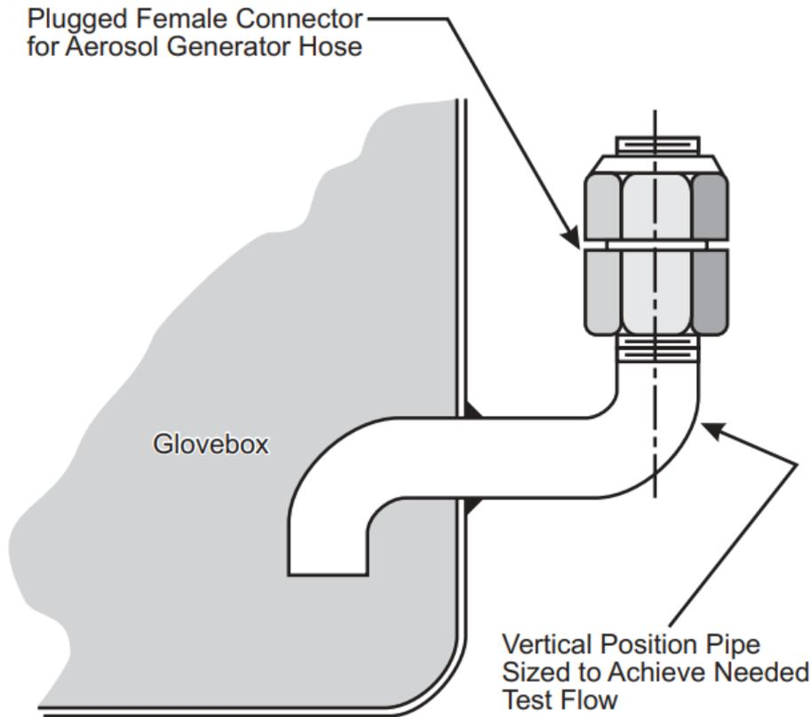
**Figure 4.22: Connection for Introducing Test Aerosol into Glovebox**
