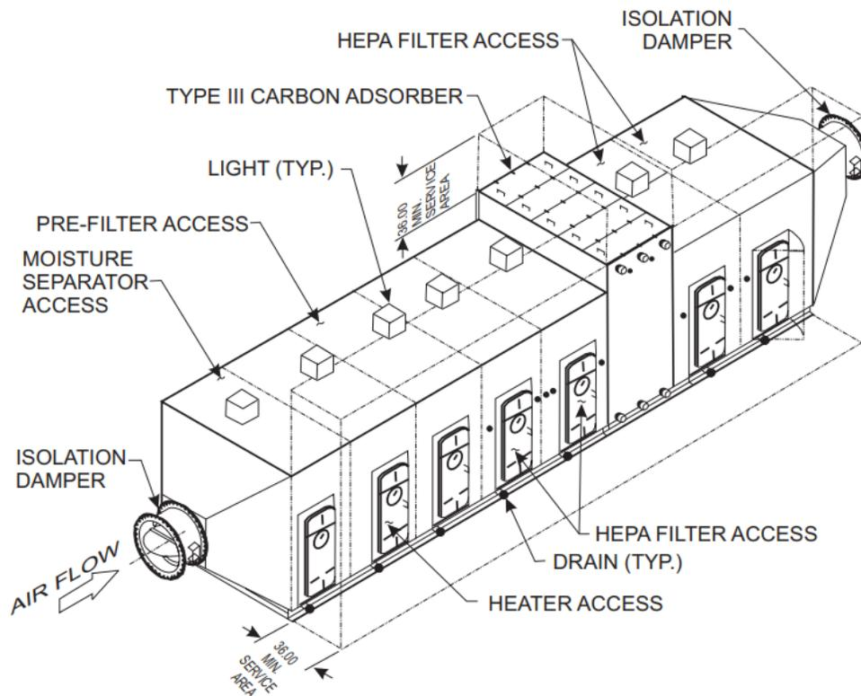
Figure 4.65: Desirable Air Cleaning Housing Features (a)
