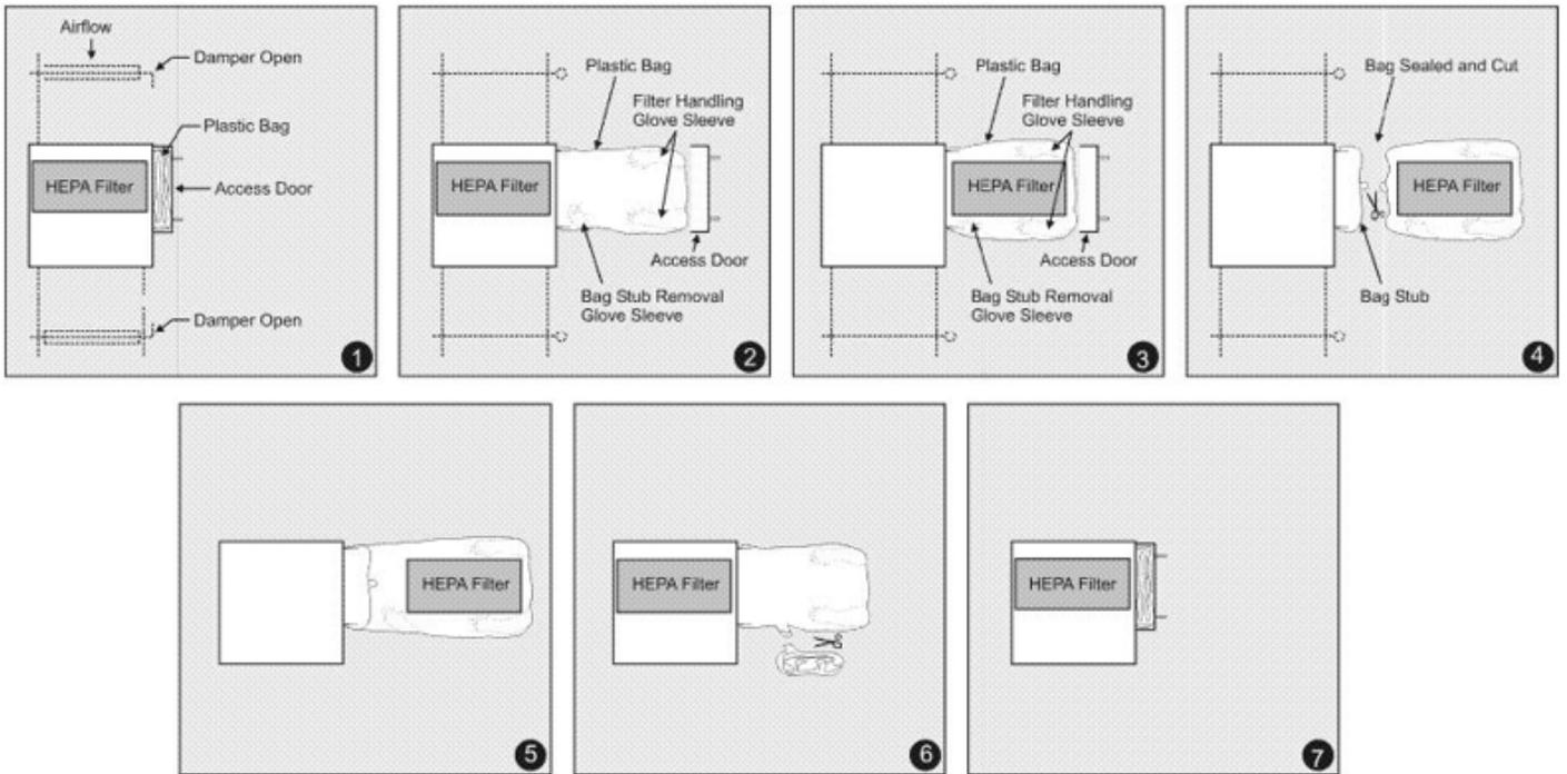
Figure 4.31: Bag-In Bag-Out Filter Replacement
