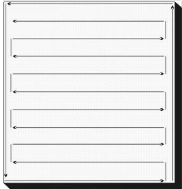
Figure 8.15 – Recommended Scanning Pattern
