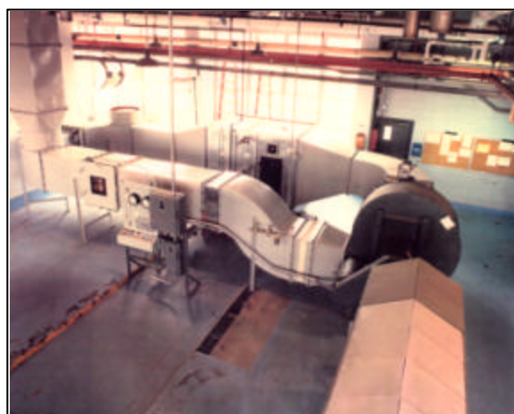
Figure 8.3 – Overpressure Resistance Tester
