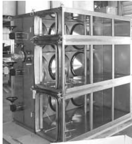
Figure 4.63 – Side-Access Housing with Multiple Inlet Valves
