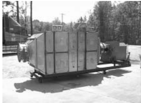
Figure 4.2 – Side-access Design (Square Filter)
