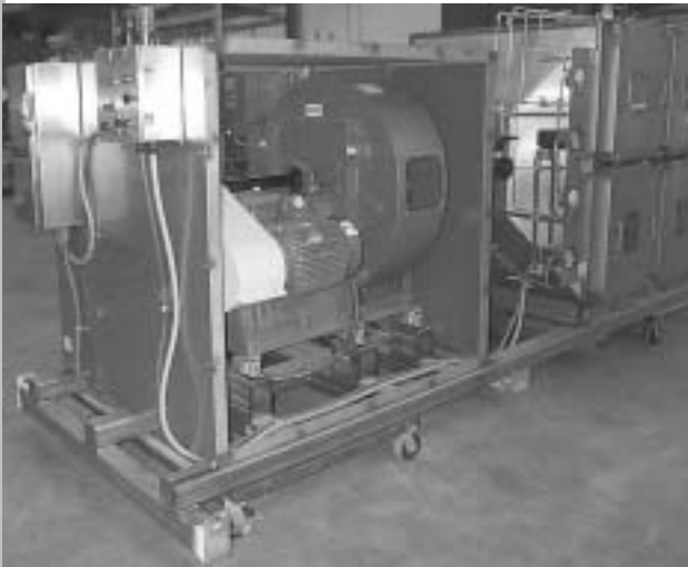
Figure 4.58 – Side-Access Housing with Fan
