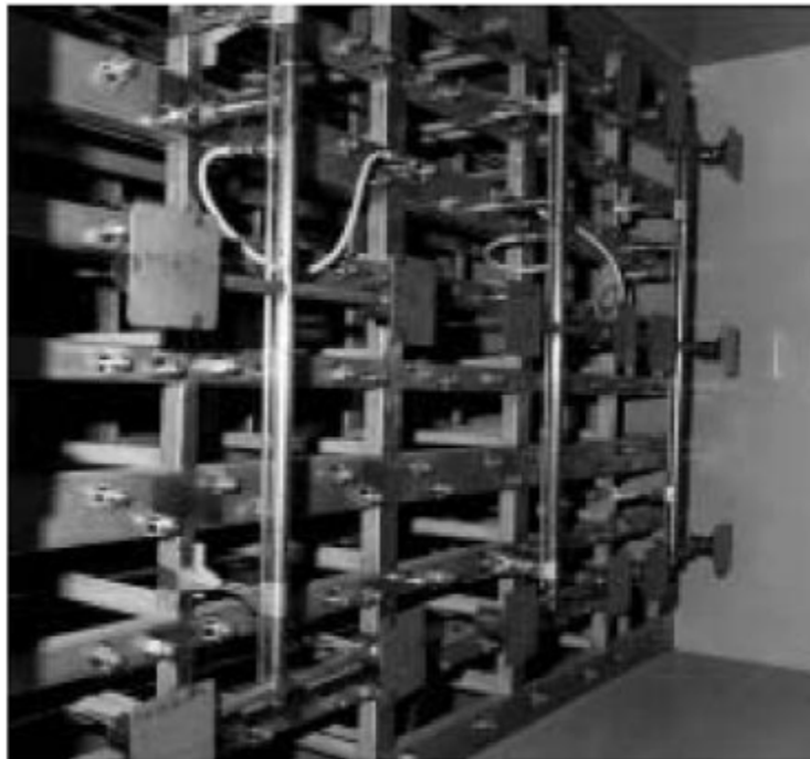
Figure 4.54: Absorber Mounting Frame with Test Section Manifold
