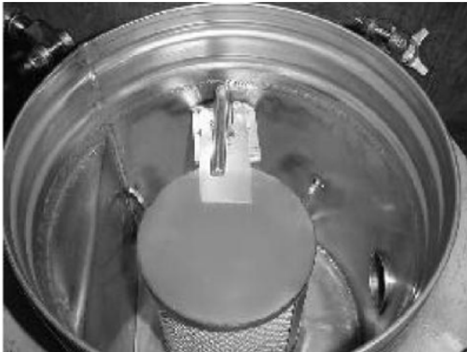
Figure 4.40: Clearance Between Radial Flow Filter and Housing
