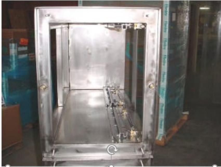
Figure 4.25: Turned Angle, Gasket Sealing Filter Surface for a Commercial Housing
