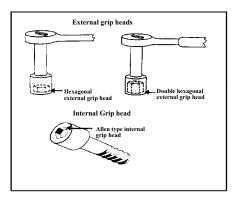
**2.11.9.4 Tool access.** Direct tool access should be provided to allow for torquing without the use of irregular extensions (See also Section 1.4, Equipment accessibility, of this document).
