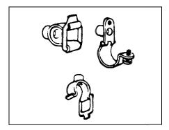
Figure 2.6.3. Quick release, hinged and spring type clamps.
