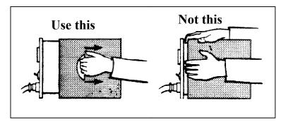
**2.13.6 Lifting criteria for handles.** Handles should meet the lifting criteria listed in Table 2.13.1, Lifting Criteria for handles.
