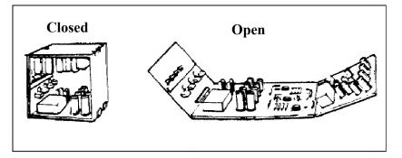
**2.2.3.7 Braces.** Braces or similar items should be provided to hold hinged assemblies in the "out" position while they are being worked on. Rests or stands should be provided to prevent damage to delicate parts. If feasible, the rests or stands should be a part of the basic chassis (See Figure 2.2.7, Bracing of hinged assemblies and Figure 2.2.8, Use of stands for component maintenance).
