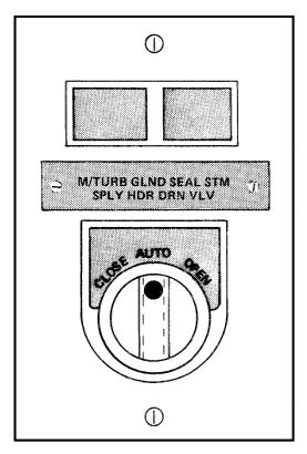
Figure 2.3.8. Relating labels to controls and displays (Ex. 1.3.11)
