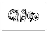
c. Reels or reel carts for handling large, heavy, or long lines or cables. Automatic rewind should be available, where possible, to minimize damage and kinking (See also Figure 2.6.5, Line and cable reel cart).
