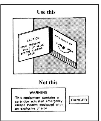
Figure 2.3.9. Examples of warning labels.
