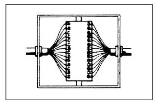
Figure 2.6.12. Cable "fanning" for ease of maintenance.
