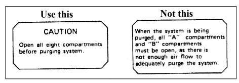
c. Labels containing a number of steps to be performed sequentially should itemize the steps rather than present them in paragraph form (See Figure 2.3.2, Label containing usable sequence of steps).
