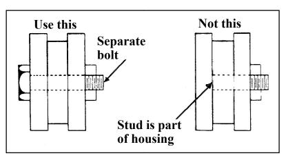
Figure 2.11.1. Example of proper and improper design of bolt fastener.
