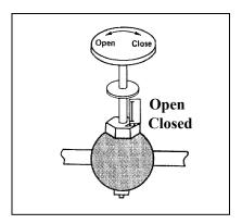
**2.5.1.7.4 Circular handles.** When circular handles are used they should have crowns or should employ concave areas or convex projections along the periphery of the handle.
