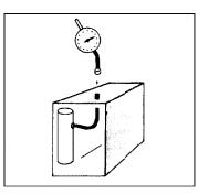
**2.8.2.3 Use of guides.** Suitable guides for test probes should be provided when test points are located internally or blind operation is required.
