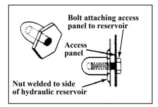
Figure 2.11.13. Example of lock nut.
