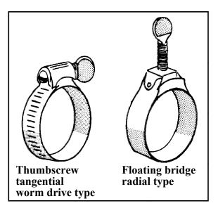
**2.11.10.3 Captive fasteners.** These are slower and more difficult to use (depending upon type), and require use of common (usually) hand tools; however, they stay in place, save the time spent handling and looking for bolts and screws, and require only one-handed operation. Captive fasteners should:
