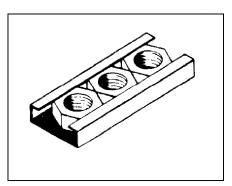
c. Only be used with nut-plates when several bolts are to be fastened on one surface and alignment is not a problem. (Nut-plates heavy and expensive to replace when a hole is stripped.)
