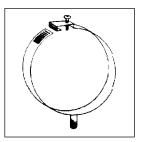
b. Only require one hand operation where more holding force is required (See also Figure 2.11.7, Example of clamp requiring one hand operation).
