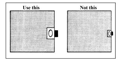
b. Along with their catches, be located and positioned so they will not open accidentally under usual operating conditions (See also Figure 2.11.5, Example of effective positioning of latches).
