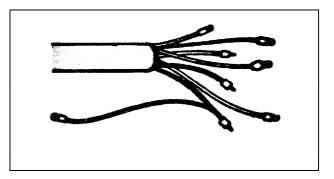
e. Where possible, use physical measures, such as cable length, to prevent interchanging units or components with the same or similar form, that are not, in fact, functionally interchangeable.
