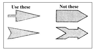
Figure 2.3.4. Use of arrows with narrow width-to-length ratios.
