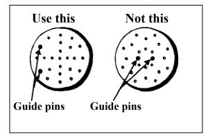
Figure 2.7.10. Example of asymmetrical aligning pin arrangement.
