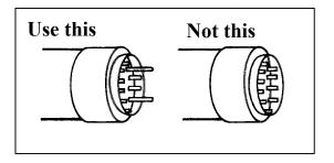
**2.7.4.3.6** Assuring alignment before electrical contact. The configuration of aligning pins, keyways and other equivalent devices should insure that alignment is obtained before the electrical pins engage and contact is made.
