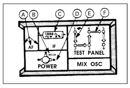
**2.2.2.12.1 Content of panel and equipment labels.** Provisions should be made for the following information and instructions to appear on system panels and equipment when appropriate (see also Section 1.3, Hardware Identification for maintainability, of this document):
