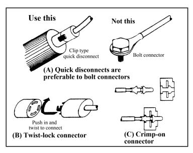
**2.7.4.3.5** Aligning pins. Plugs should be used in which the aligning pins or keys extend beyond the electrical pins. This arrangement protects the electrical pins from damage through poor alignment or twisting of the plug when it is partially inserted (Figure 2.7.9, Example of extended alignment guides).
