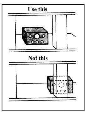
Figure 2.2.2. Proper placement of components.
