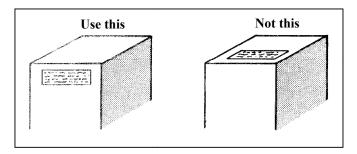
Figure 2.3.6. Component labeling to preclude operating error.
