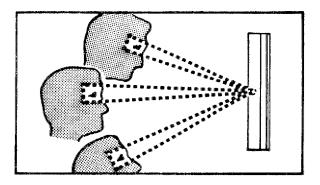
**2.5.2.15 Direct-reading type indictors.** Where possible, direct-reading type indicators should be used for hydraulic and other fluid tanks. For example, to facilitate quick visual inspection of the presence of oil in gear cases, oil level sight plugs may be used. This eliminates the need for dipsticks or fluid level gauges (See also Figure 2.5.9, Oil level sight plug).
