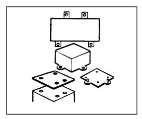
**2.2.3.4 Interchangeable components**. Components with the same form, function, value, and reliability and other requirements should be completely interchangeable throughout the system or related systems.
