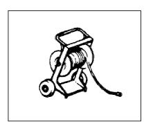
Figure 2.6.5. Line and cable reel cart.
