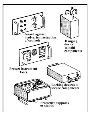
Figure 2.13.6. Examples of miscellaneous uses for handles.
