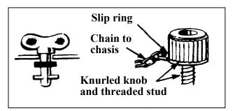
**2.11.10.4 Combination head-bolts and screws.** These should be used in preference to other screws or bolts simply because they may be operated more rapidly with either a wrench or a screwdriver. This allows use of the more convenient tool and reduces the possibility of slot damage and stuck fasteners. In general, slotted, hexagonal heads are preferable to knurled and slotted heads (See also Figure 2.11.9, Examples of combination head bolts and screws and slotted hexagon screws).
