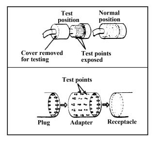
**2.7.4.3.12** Number of pins. Fewer plugs with many pins should be used rather than many plugs with few pins. It takes about the same amount of time to connect a plug with many pins as it does one with few pins (See also Figure 2.7.14, Example of proper use of plugs with many pins).
