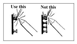
e. Terminals or other connections to which wires are soldered should be made long enough so that insulation and other materials are not burned by the hot soldering iron (See also Figure 2.6.11, Proper length of terminals and connections).
