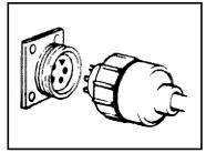
**2.7.3.6 Soldering, brazing, or welding.** Such methods provide the securest connection and are often the most efficient way of securing small connection points or maintaining hermetic seals, but such connections require considerable maintenance time for connection or disconnection. These connections should meet the following criteria:
