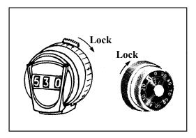
Figure 2.5.4. Tool actuated control.
