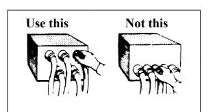
Figure 2.7.11. Proper arrangement of electrical connectors.
