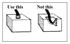
**2.7.4.3.11 Integral test points.** Plugs should be used with integral test points for each input and output that cannot be easily checked. Otherwise, an integral sliding cover for the test points in the plug should be provided if dust and moisture is a problem. As an alternative, a test point adapter may be provided for insertion between plugs and receptacles (See also Figure 2.7.13, Examples of plugs with integral test point or test point adapter).
