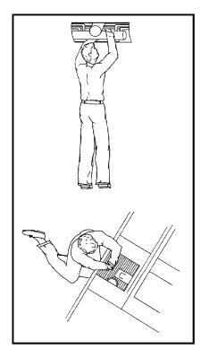
**2.4.9 Routing systems to allow use of lifting and movement aids.** Systems should be routed around access paths and envelopes such as overhead cranes, other movement paths and equipment-hatch removal envelopes. Overhead clearance should be a minimum of 2.13 m (7 ft) above the floor for passage of personnel and removal of equipment. Where applicable, sufficient clearance should be provided to permit the use of vehicular or other transportation aids near the system.
