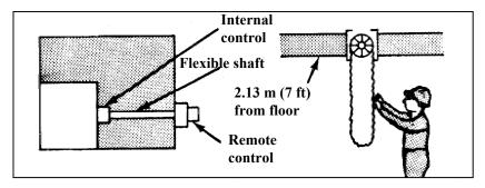
**2.5.1.3 Emergency controls.** Emergency controls which may be operated by the maintainer should be located so that they may be activated from any position in the maintenance work area. if the work area is especially large and access to a single emergency control is difficult, duplicate controls should be provided.
