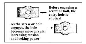
Figure 2.11.14. Example of a clinch nut.
