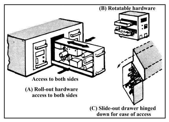
Figure 2.12.1. Examples of drawer and rack design.
