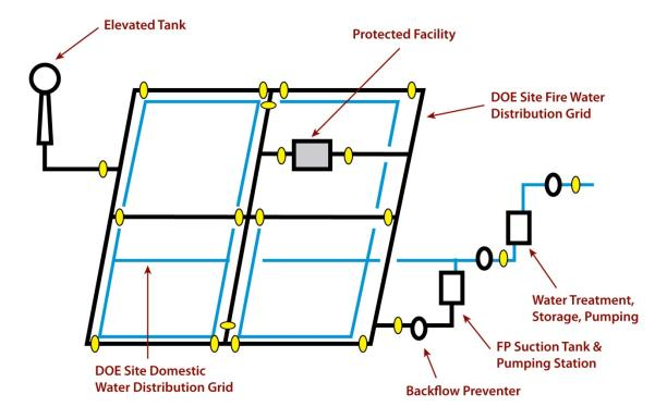
Similar to Arrangement 2, this arrangement should not be used for SC applications, but is used for general purpose fire protection and may be used for SS applications, if requirements for reliability, QA, and safe operation are met. The reason the system is not to be used in SC applications is that, even though the system is under DOE control, it is not under the facility's control. Thus having an additional backup system that is under the facility's control is prudent.
