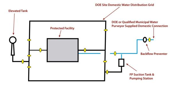
This arrangement could be used for SS applications, if conditions specified in A.3.2 and A.3.3 of Appendix A are met. If the supplied sprinkler system is required for mitigation of a seismically-induced fire, the supply system shall be categorized as SS.
