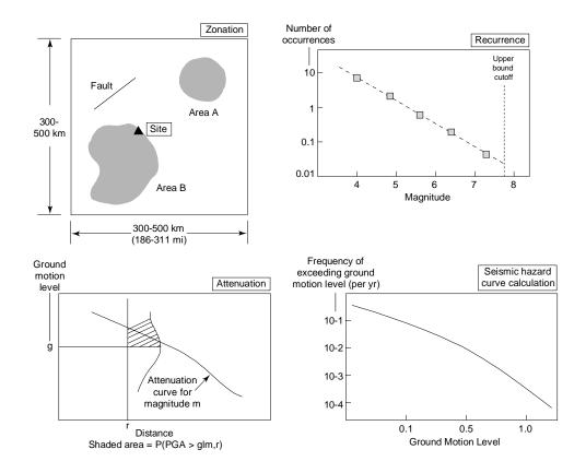
Figure 3.1 Four Steps in Probabilistic Seismic Hazard Analysis
